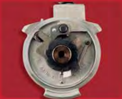
RA Model (pg.59) Ratchet and Pawl Design
