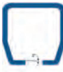
The 2° taper of the running flange helps to center the trolley in the track for smooth, effortless movement of trolleys and end trucks.
