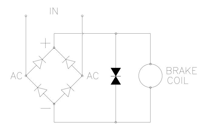
TYPICAL SCHEMATIC 120-575VAC INPUT
