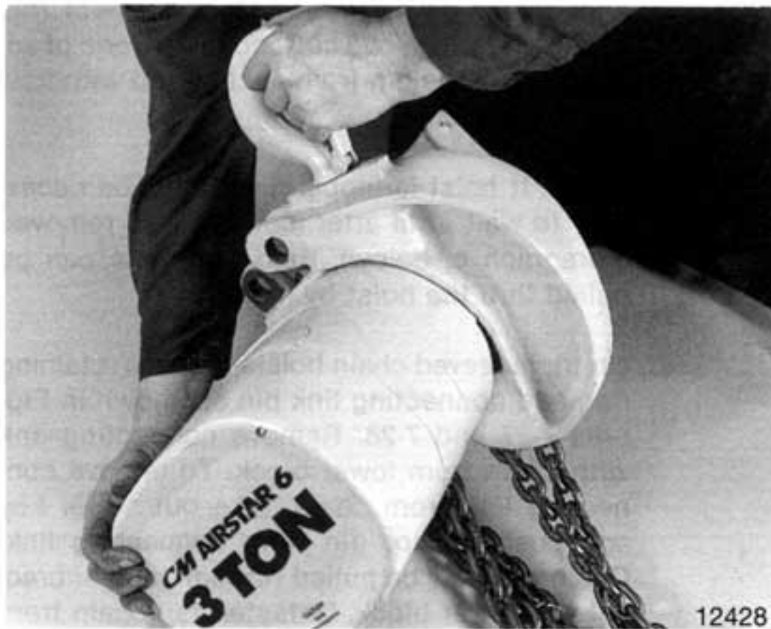
Figure 7-2. Removing 3 Ton Hanger Bracket from Hoist Frame.
