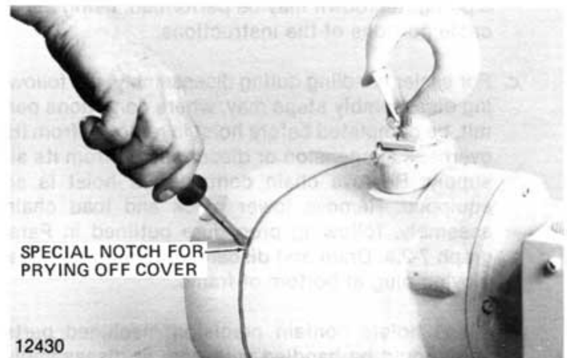
Figure 7-4. Prying Gearcase Cover From Hoist Frame.
