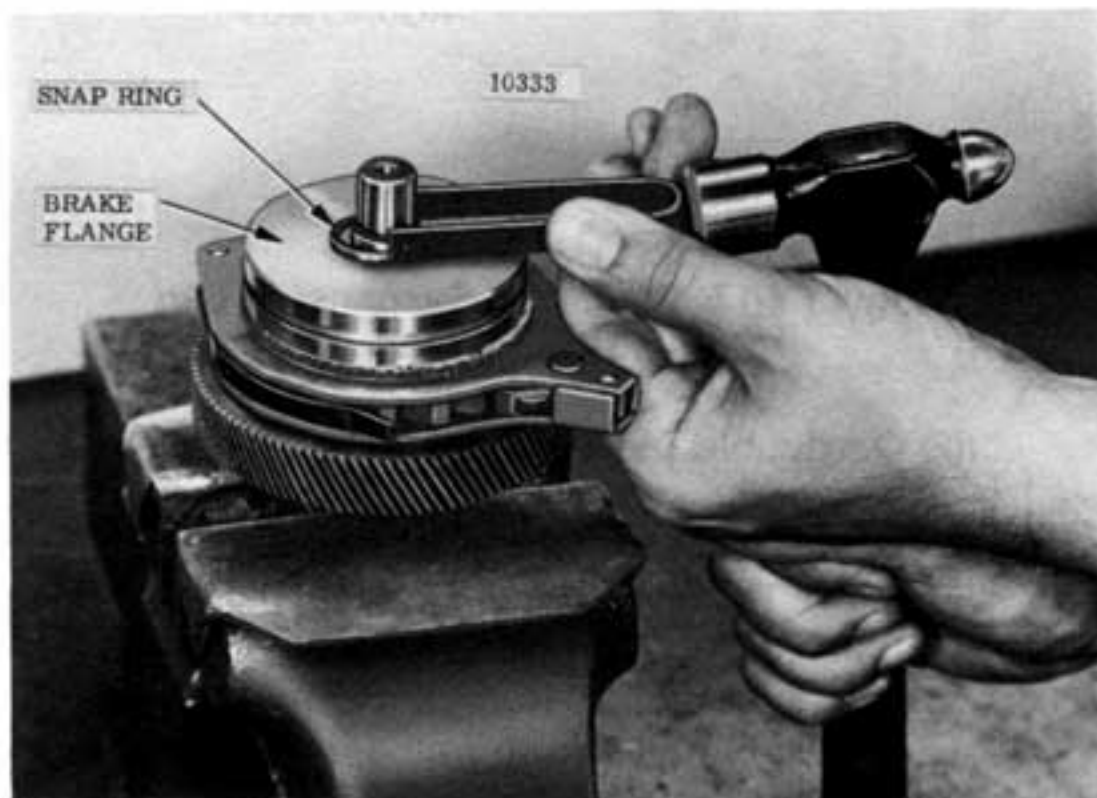
Figure 7-18. Removing Snap Ring from Load Brake Shaft.
