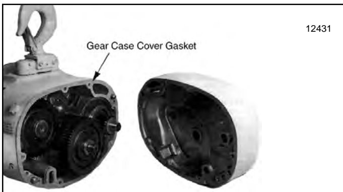
Figure 7-5. Gearcase Cover Removed From Hoist Frame
