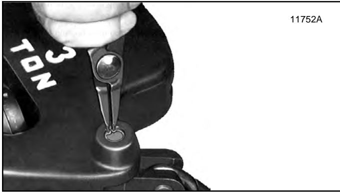
Figure 7-27. Removing Retaining Ring From Bore of Connecting Link Pin - Triple Reeved Lower Block Assembly
