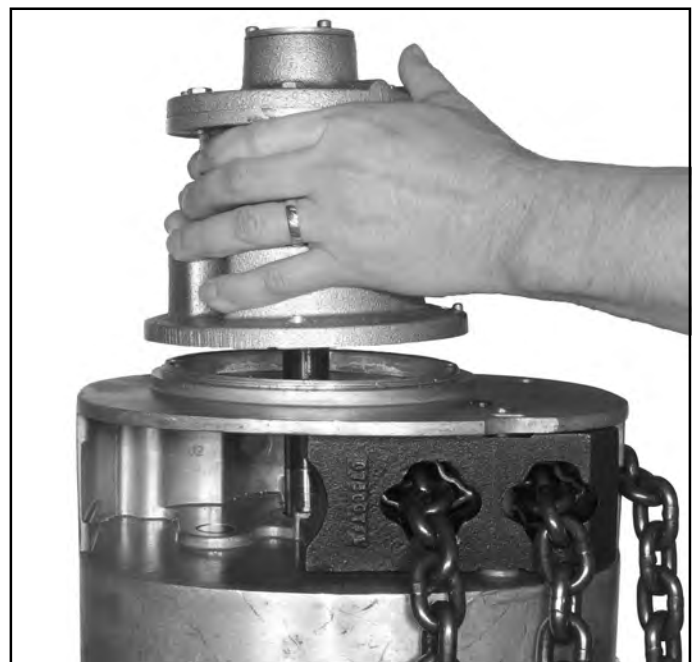
Figure 7-8. Removing Motor Assembly
