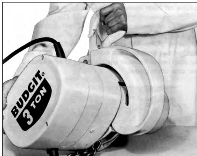
Figure 7-3. Removing 3 Ton Hanger Bracket from Hoist Frame
