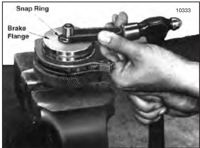
Figure 7-21. Removing Snap Ring from Load Brake Shaft
