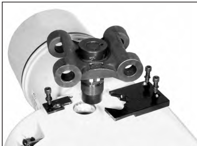
Figure 7-20. Removing Suspension Lug (1/4 through 1 Ton Models)
