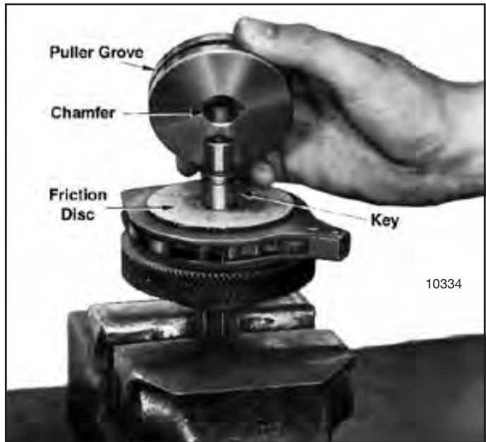
Figure 7-22. View Showing Load Brake Flange Removed
