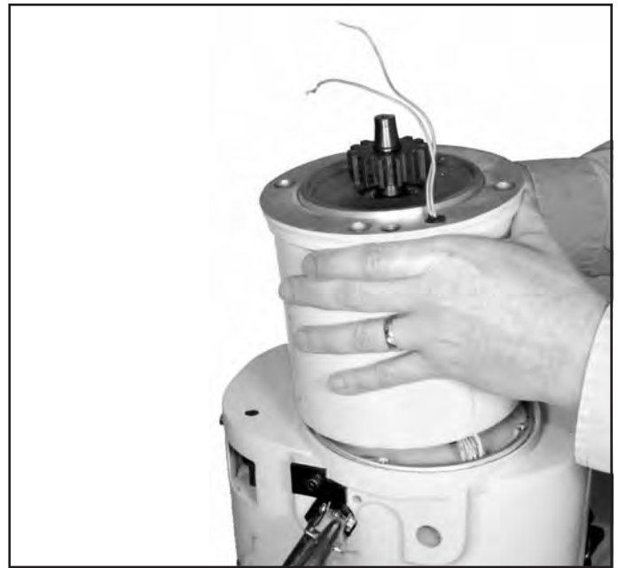
Figure 7-9. Removing Motor Assembly
