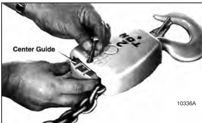
Figure 7-27. Removing Chain Center Guide from 2 through 5 Ton Lower Block Assembly
