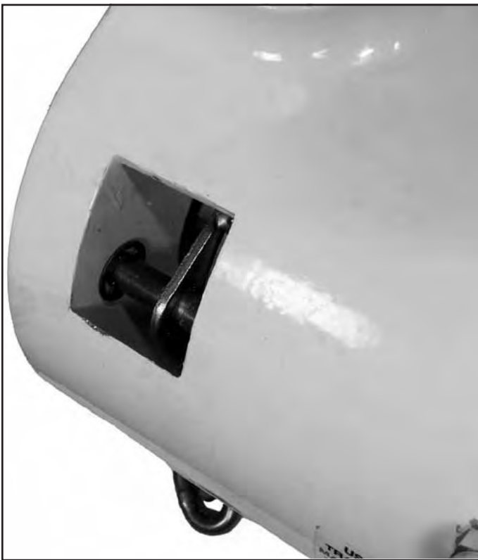
Figure 7-13. Removing Chain Guide Support Pins
