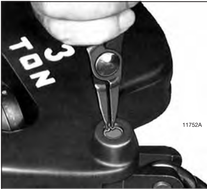
Figure 7-30. Removing Retaining Ring from Bore of Connecting Link Pin - 3 Ton Lower Block Assembly
