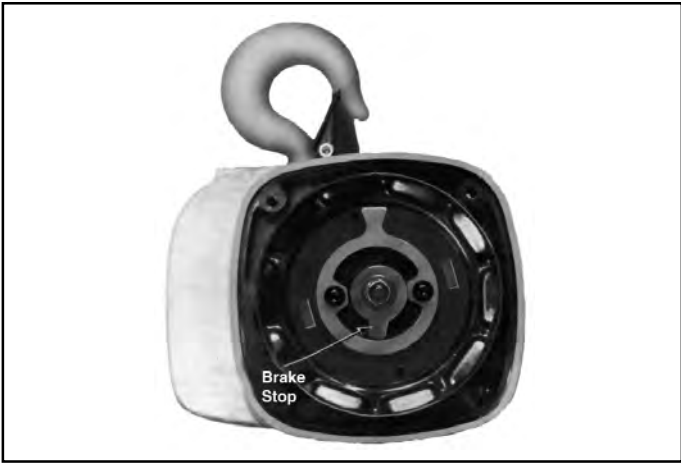
Figure 7-6. Brake Stop Position for 1/4 and 1/2 Ton Models
