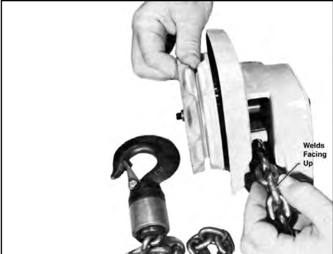
Figure 7-8. Installing Load Chain
