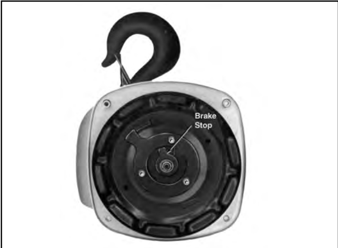
Figure 7-7. Brake Stop Position for Other Models
