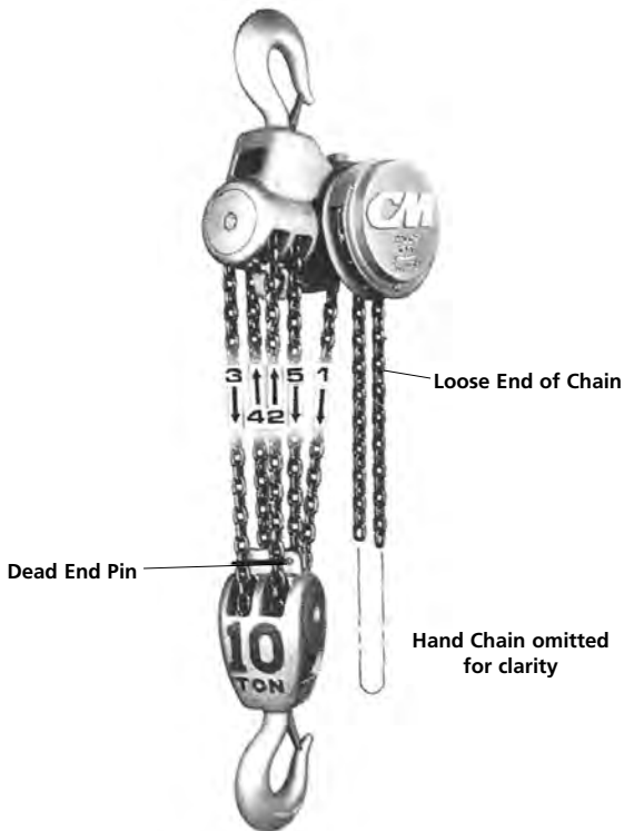
FIGURE 21. Reving 10 Ton Hoists
