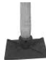
Close Up of Tamper
