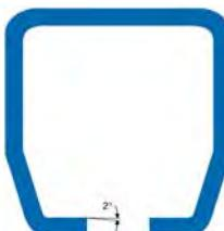
The 2° taper of the running flange helps to center the trolley in the track for smooth, effortless movement of trolleys and end trucks.
