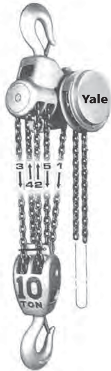
FIGURE 21. Reeving 10 Ton Hoists
