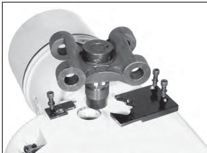
Figure 7-20. Removing Suspension Lug (1/4 through 1 Ton Models)
