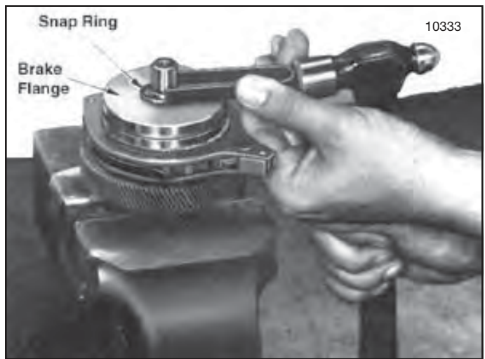
Figure 7-21. Removing Snap Ring from Load Brake Shaft
