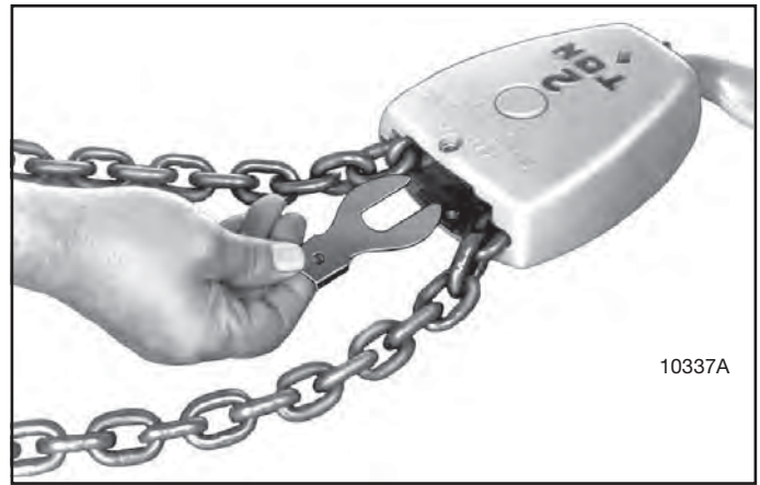
Figure 7-28. Removing Sprocket Pin Lock on 2 through 5 Ton Lower Block Assembly
